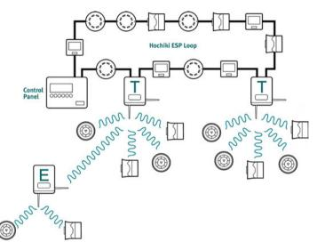
The RSM-WTM Translator Module (T) is fitted to the analogue addressable fire system loop. It then provides an interface between the loop and the wireless devices. The module is fully powered by the loop and full control and monitoring of the wireless devices is possible through the control panel.
